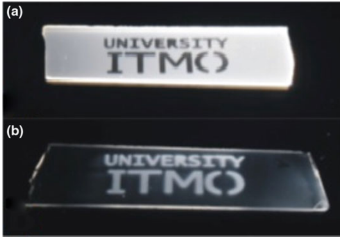
Fig. 5.23 Negative and positive luminescent images in PTR glass plates irradiated through the mask by the UV nanosecond laser radiation with (a) and without (b) the preliminary irradiation by the UV mercury lamp [29]
