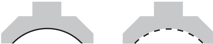
FIGURE 7.20 Cross-sectional view of two different types of spherical cup wheels used for fine grinding with bound abrasive grains; cup wheel with closed abrasive coating (black line, left), and cup wheel with abrasive pellets (black structures, right).
