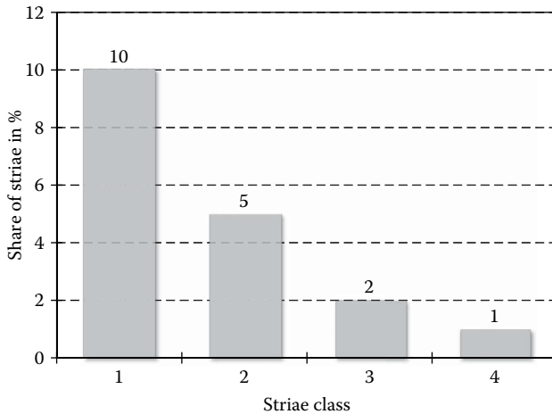
FIGURE 6.3 Striae classes 1–4 including the particular percentaged share of striae in total optically active surface area of an optical component. (From Schott, A.G., Optical Glass Data Sheets, 2015.)
