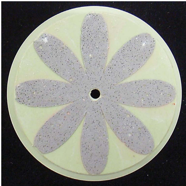
FIGURE 8.6 Polishing tool with blossom-like structured polishing pad made of polyurethane.
