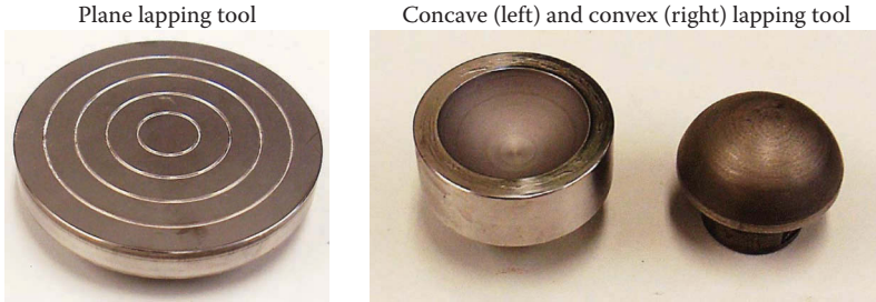
FIGURE 7.23 Examples for lapping tools made of gray cast iron used for loose abrasive grinding.
