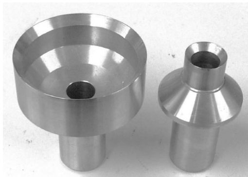
FIGURE 10.4 Examples for clamping bells of different diameters.
